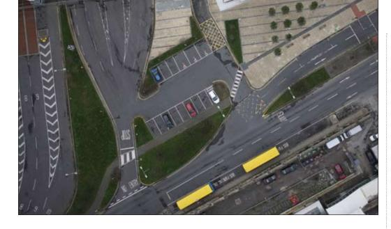
ground markers to provide photo control. The GPS unit has an expected spatial accuracy when operated in the subject region of 10-25mm.
