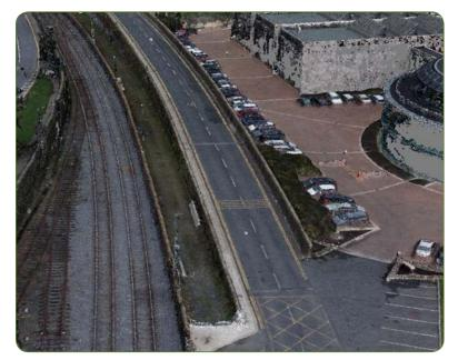
Fig. 6: 3D point cloud has 2 cm absolute accuracy.
